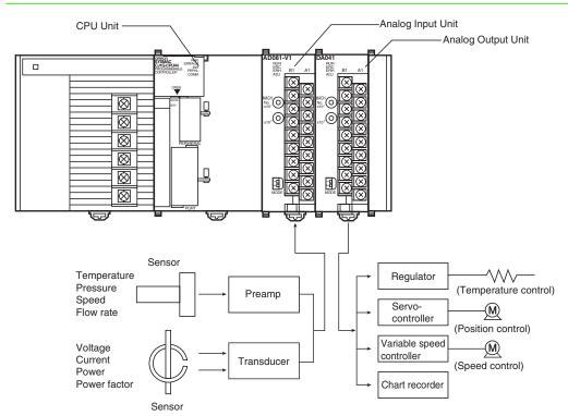
Note: The above diagram is an installation example for the CJ1W-AD081-V1 Analog Input Units and CJ1W-DA041 Analog Output Units.
