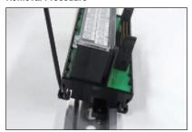
1.Insert a flat-blade screwdriver into the DIN Track lock. 2.Move the screwdriver like a lever to free the lock.
