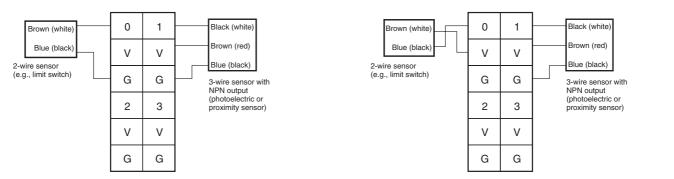
Note: Wire colors have been changed according to revisions in the JIS standards for photoelectric or proximity sensors. The previous colors are given in parentheses.
