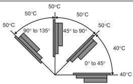
**\*2.** Use the Programmable Terminal within the following temperature and humidity ranges.
