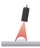
\*\*When inclination is great, a measurement error may occur. Check the measurement accuracy in actual measurement conditions prior to use.
